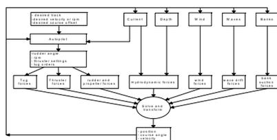
Flow diagram of the SHIPMA model
